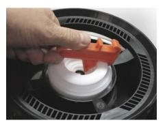
Polykegs require an orange de-gas key. Angle as per the diagram and press down into the centre of the keg.
