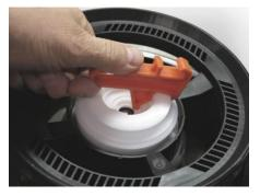
Polykegs require an orange de-gas key. Angle as per the diagram and press down into the centre of the keg.
